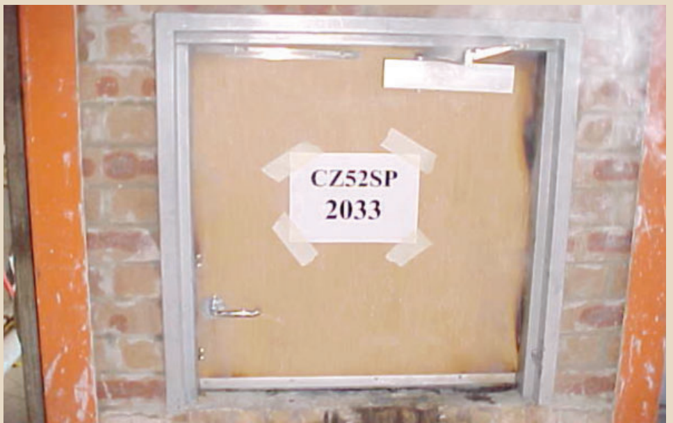
Photo of some perimeter and automatic door seals being fire tested on a small scale (pilot scale) furnace – Courtesy of Lorient Australia
