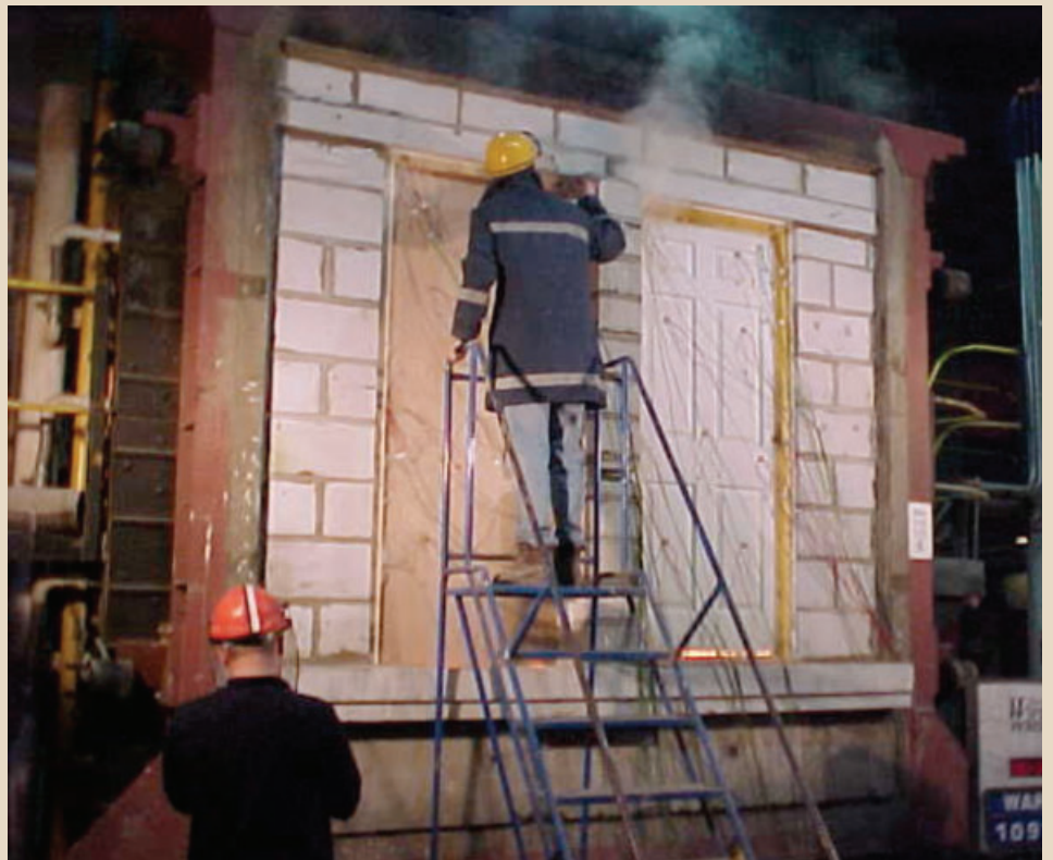
Photo of a full scale fire resistance test on a pair of single fire resistant doorsets
