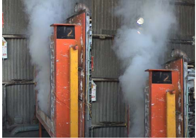
Smoke leakage during testing of tight fitting fire door
