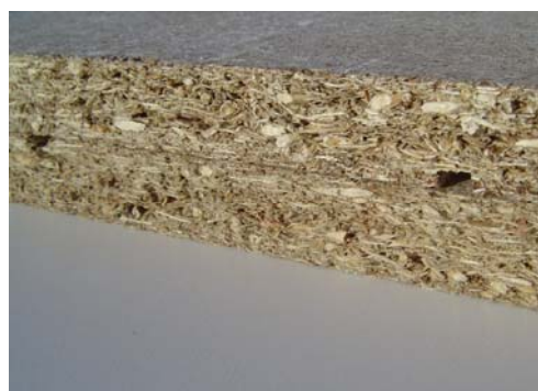
Cellulosic (timber) based core material
