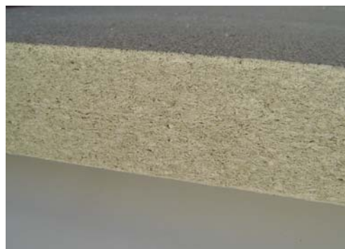
Mineral fibre based core material
