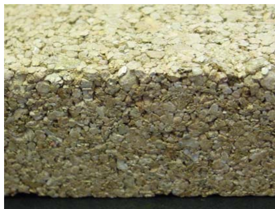
Vermiculite based core material
