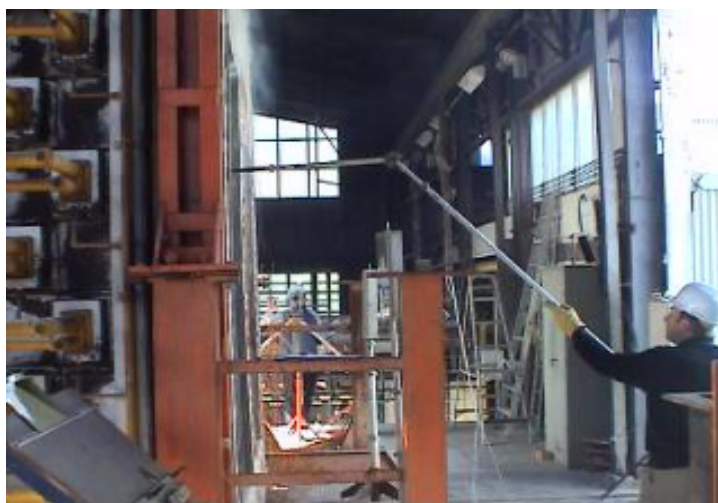
Deflection measurements being taken during a fire test
