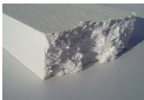
Calcium silicate based core material
