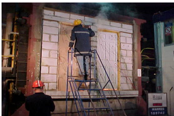
Photo showing typical full scale fire test on two single leaf door assemblies in a masonry wall construction
