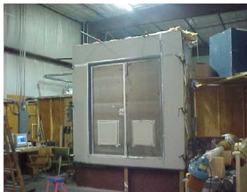
Smoke door being tested to AS 1530.7
