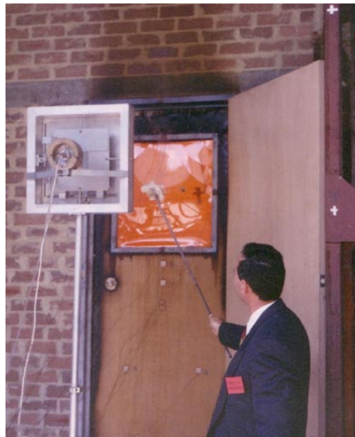
Fire door testing incorporating a vision panel
