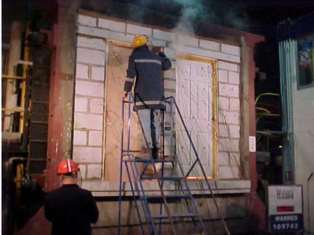
Photo of a full scale fire resistance test on a pair of single fire resistant doorsets
