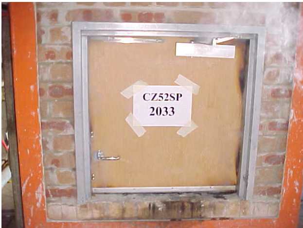
Photo of some perimeter and automatic door seals being fire tested on a small scale (pilot scale) furnace – Courtesy of Lorient Australia
